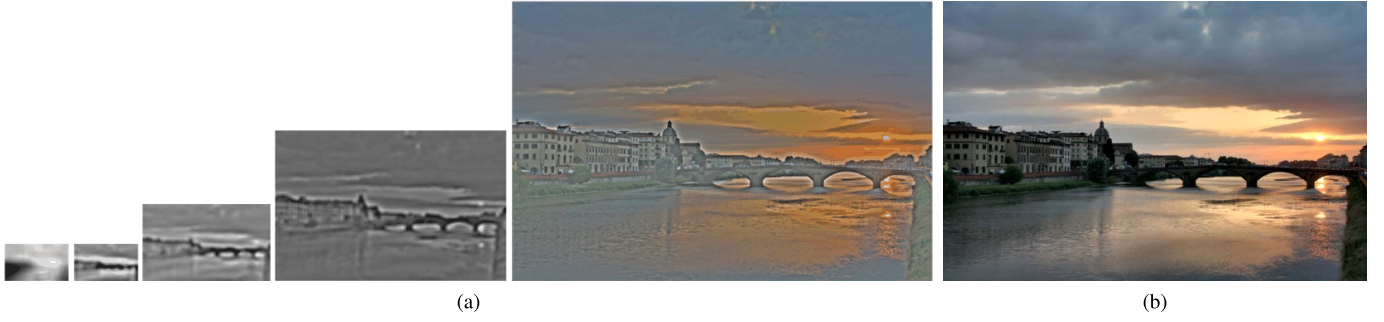
Fig. 5. Visual demonstration of the proposed multi-scale SPD-MEF approach on the image sequence “Arno” (courtesy of Bartłomiej Okonek). (a) Desired base and detail layers at four scales. (b) Final fused image.
