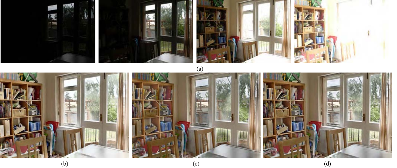
Fig. 9. MEF-Net in comparison with its variants. (a) Source sequence “House” courtesy of Tom Mertens. (b) Guided filtering as post-processing. (c) Bilinear upsampling trained end-to-end. (d) MEF-Net (guided filtering trained end-to-end).
