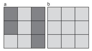
**Fig. 2.** The normal case (a) versus singular case (b) when calculating estimating values (dark gray area represents pixels in **E** and light gray area represent pixels belonging to **I**).
