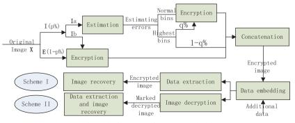
Fig. 1. The framework of proposed method.
